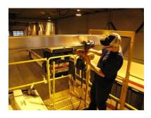
10) Lift hoist into position and hook it onto trolley.
