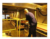
9) Remove lower bolt on end stops and roll trolley onto "I" beam. Reinstall and tighten end stop bolts to prevent trolley from coming off of "I" beam. Remove hoist from storage position.
